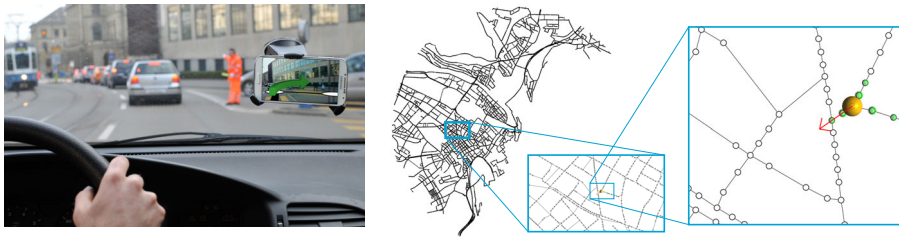
Fig. 1. A device capturing images at low frame rate is mounted on a car driving around an urban environment. Our approach exploits the captured images and the streetview graph to track the movement of the vehicle on the map.
